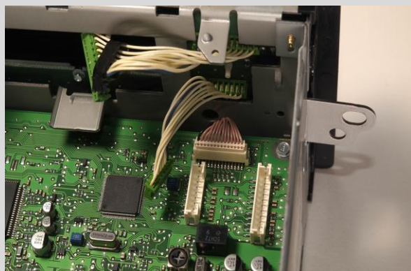
Two connectors unfastened from the top PCB board
