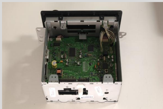
Placing the metal plate aside, PCB board and its connectors is accessible
