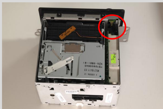
The bottom of the radio has a third connector that needs to be unfastened
