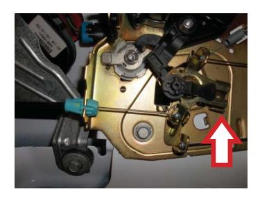
**STEP 2:** Attach the lift gate lock actuator into position.
