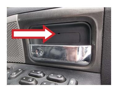
**STEP 2:** Using a 10mm socket and ratchet assembly, remove the interior door trim panel retaining screws.
