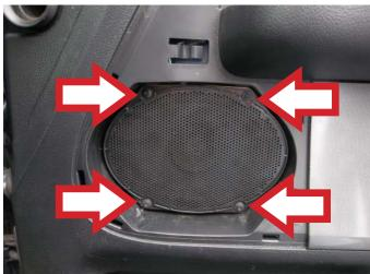
**STEP 13:** Install the speaker bezel assembly. **NOTE:** Be sure to align the bezel assembly retainers with their corresponding holes. Failure to do so will cause damage to the speaker bezel assembly.
