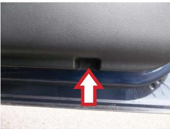
**STEP 4:** Using a trim panel removal tool, release the speaker grille assembly.
