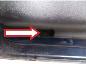
**STEP 15:** Using a 10mm socket and ratchet assembly, install the two (2) interior door trim panel retaining screws.
