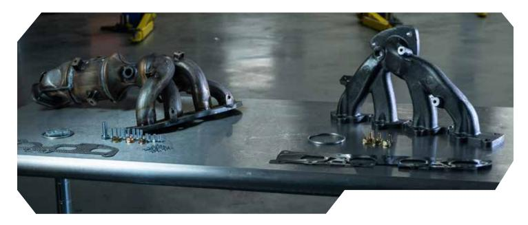
Install our replacement **catalytic converters** with confidence, especially when chasing PO420/ PO421 codes. Fully CARB compliant, these end the constant tradeoff of questionable design and function just for low price. You can have both! Dorman upgrades traditional **cast manifolds** by upgrading construction from grey iron to ductile (nodular) cast iron, which offers greater fatigue resistance and strength, as well as increased flexibility through inevitable heat cycling.
