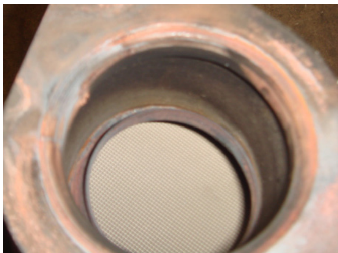
Normal converter coloration indicating proper combustion
