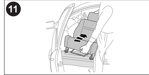
Install seat - apply proper torque on all seat fasteners. Make sure seat track is clear and all seat height and seat back adjustments are free to move.
