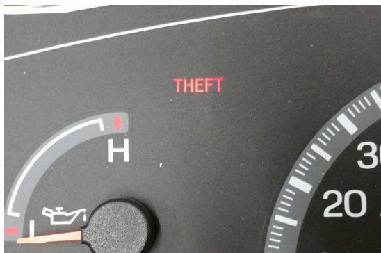
Cluster with NO Tachometer – theft light location
