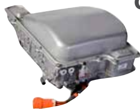
Drive Motor Inverters
