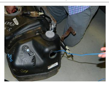
**STEP 10:** Remove pull wire after the outer gasket and locking ring are on.
