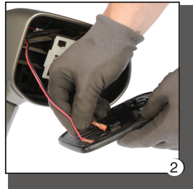
Fig. 2. Reconnecting the mirror glass assembly. A. If vehicle has a heated mirror, connect the wires to the heater terminals.
