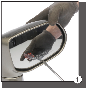
Fig. 1. Removing the broken mirror glass assembly from the current housing.
