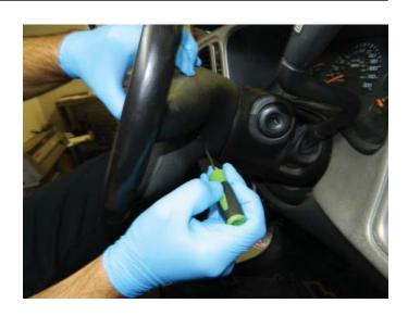
STEP 5: Remove steering wheel airbag.
