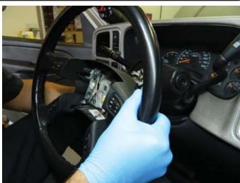
**STEP 9:** Using a flat-blade screwdriver, pick, or other non-marring tool, release the upper and lower steering column covers.
