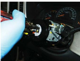
**STEP 7:** Remove the orange stop clip from the clock spring.
