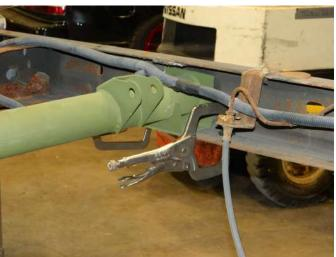
**STEP 8:** Using a permanent marker, mark off the section of the frame around where the crossbar attaches to the frame, so you can clean down to the bare metal for a proper and strong weld.
