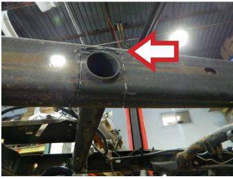
**STEP 4:** Using a cutting wheel, cut the bed support from the crossbar.
