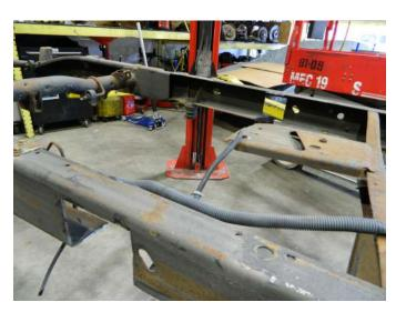
**STEP 6:** Place the replacement crossbar in place of the removed one.
