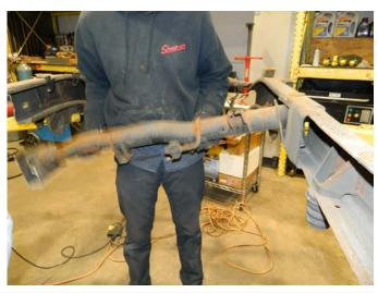
**STEP 6:** Place the replacement crossbar in place of the removed one. Hold the replacement crossbar in place to the frame with c-clamps or vice grips. Then, using a permanent marker, mark off the section of the frame around where the crossbar attaches to the frame (on both sides of the frame).
