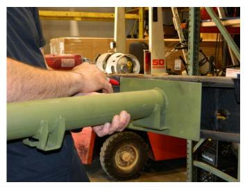
**STEP 12:** Remove the tube and inner plates from the frame. Then, using a flap wheel disc, sand the inside of the frame to clean for welding, on both sides of the frame.
