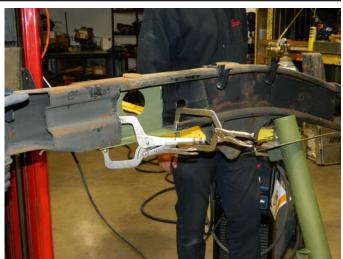
**STEP 10:** Using a welding torch, weld the outer plate to the outside of the frame on both sides of the crossbar.
