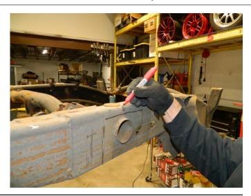
**STEP 4:** Using a cutting wheel, finish cutting around the bottom and inside of the ends of the crossbar on the frame, on both sides of the frame. Once complete, the cut will go up and over the tube on the outside and inside of the frame, on both sides of the frame.
