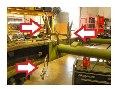
**STEP 15:** Using a welding torch, weld the inner plate to the inside of the frame, on both sides of the frame. Then, weld around the tube to the inner and outer plates, on both sides of the frame.
