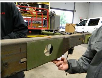
**STEP 7:** Remove the replacement crossbar and the c-clamps or vice grips. Then, using a handheld torch and paint scraper, clean down to the bare metal where the crossbar will attach to the frame, on both sides of the frame, for a proper and strong weld.
