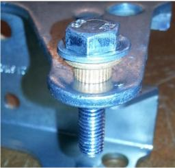
Step 3 – Install two washers [Option 2] on to the bolt (once the assembly is inserted on the hinge bracket bore (pictured above)). Next insert one washer [Option 1] and install the nut until the assembly is hand tight as pictured below (please make sure that the bushing, hinge bore, and washers are as concentric as possible in order to allow for proper installation).
