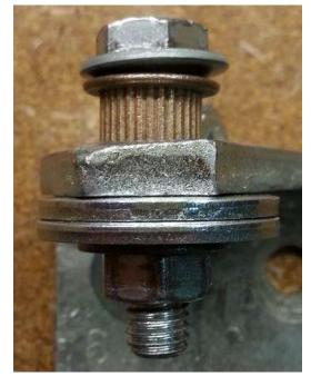
Step 4 – Use the crescent wrench to secure the nut at the bottom of the assembly. Proceed to ratchet the head of the bolt with the socket wrench while holding the crescent wrench securely. Only need to ratchet the head of the bolt until the flange of the bushing is flush to the hinge. DO NOT OVERTIGHTEN THE ASSEMBLY AS THIS CAN LEAD TO THE FORMATION OF CRACKS IN THE BUSHING. This process will draw the bushing into the bore to ensure the bushing is proper installed. See below:
