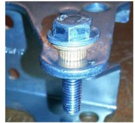
Step 3 – Install two washers [Option 2] on to the bolt (once the assembly is inserted on the hinge bracket bore (pictured above)). Next insert one washer [Option 1] and install the nut until the assembly is hand tight as pictured below (please make sure that the bushing, hinge bore, and washers are as concentric as possible in order to allow for proper installation).
