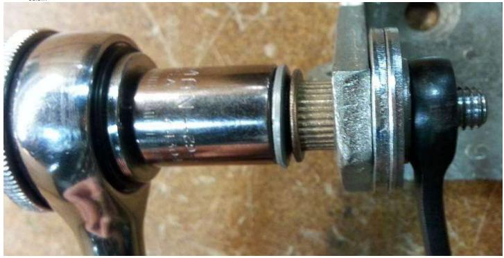
Step 5 - Remove the installation assembly. Bushing should be press fit and snug into the bore of the hinge.
