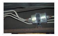
Dorman Brake Lines are made with upgraded high quality stainless steel that resist corrosion providing you and your customers a part that will outlast the OE.
