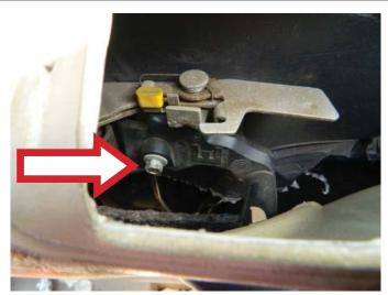
**STEP 9:** Remove the door handle assembly through the door trim panel opening.
