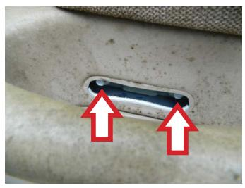
**STEP 6:** Using a trim panel removal tool, remove the interior door trim panel. **NOTE:** You may want to use a plastic trim panel tool to prevent scratching the painted surface.
