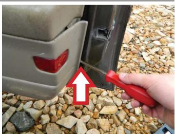
**STEP 7:** With the interior door trim panel removed from the door, disconnect the master power switch assembly. **NOTE:** The switch connectors may vary.
