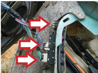
**STEP 8:** Connect the master power switch assembly.
