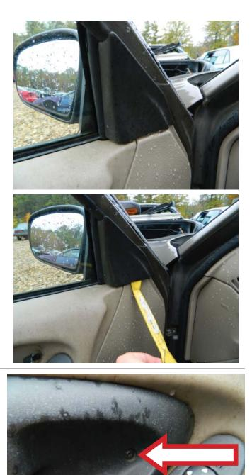
**STEP 2:** Remove the Phillips head screw attaching the interior door handle bezel assembly to the door.
