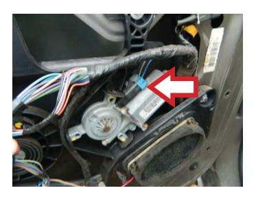
**STEP 15:** Remove the window regulator assembly attaching screws.
