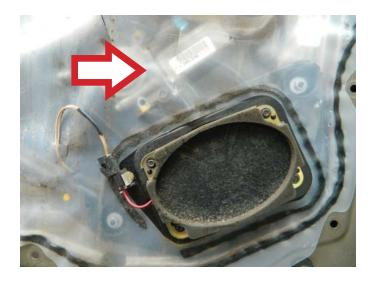
**STEP 6:** Attach the water vapor barrier.
