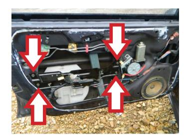
**STEP 8:** Temporarily install the master door switch to lower the window glass, exposing the window glass to window regulator attaching screws. **NOTE:** There are two (2) screws that attach the door glass to the window regulator.
