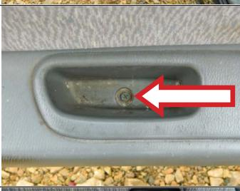
**STEP 2:** Using a trim panel removal tool, remove the master door switch assembly.
