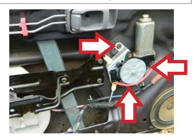
**STEP 13:** Remove the window regulator assembly through the main access hole. **NOTE:** At this point, your interior door trim panel reinforcement bracket would be removed.
