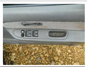
**STEP 11a:** Attach the door cup pull attaching screw.
