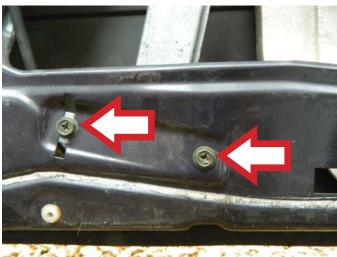
**STEP 4:** Tighten down the window lift motor attaching hardware.
