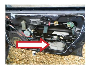
**STEP 2:** Connect the window lift motor connector.
