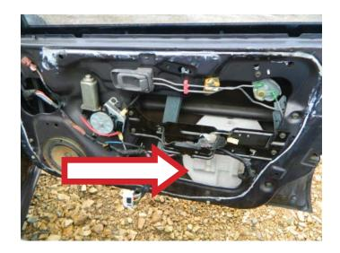
**STEP 14:** Remove the three (3) window lift motor attaching screws.
