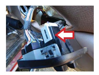
**STEP 8:** Connect the door mounted courtesy lamp. **NOTE:** Not all vehicles came equipped with a courtesy lamp. Some vehicles were equipped with a reflector.
