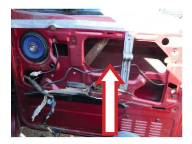
**STEP 10:** Remove the three (3) window lift motor attaching screws and remove the window lift motor from the window regulator.
