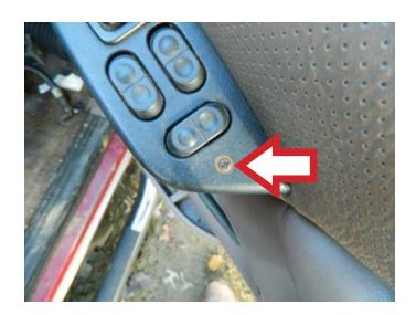
**STEP 12:** Verify that all of the interior door trim panel attaching screws are mounted securely and that the window is operating properly.
