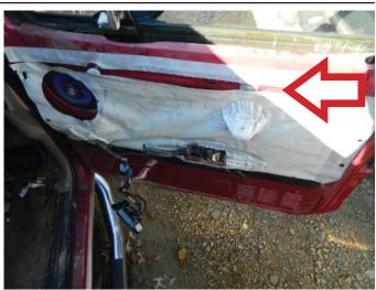
**STEP 6:** Place the master power switch assembly through the opening of the interior door trim panel.
