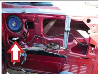
**STEP 6:** Using a ½" drill bit and a power drill, drill out the two (2) rivets holding the door brace onto the door. **NOTE:** You are using the drill and drill bit to remove the head of the rivet. DO NOT DRILL ALL THE WAY THROUGH. YOU WILL DAMAGE THE DOOR AS WELL AS THE BRACE.
