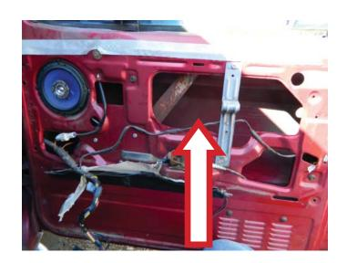
**STEP 2:** Install the window regulator onto the door and connect the window lift motor connector. **NOTE:** If you do not have access to a large rivet gun capable of handling ¼" x ¾" rivets, it is okay if you use ¼" x 20 x up to 1" bolts washers and the corresponding nylon locking nuts when installing the window regulator onto the door.
