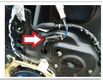
**STEP 12:** Push the window lift motor connector through the access hole in the door.
