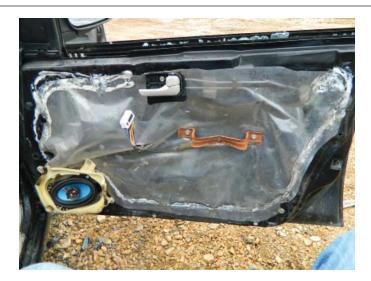
**STEP 9:** Temporarily install the window switch to lower the window glass, exposing the window glass to window regulator attaching screws.
