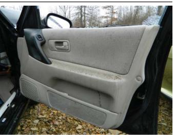
**STEP 12:** Attach the interior door trim panel attaching screws.
