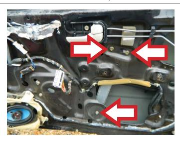
**STEP 15:** Remove the window regulator assembly through the main access hole.
