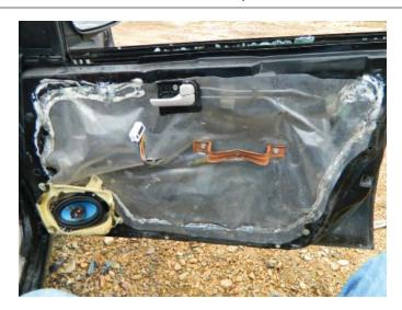
**STEP 8:** Attach the interior door trim panel reinforcement bar.
