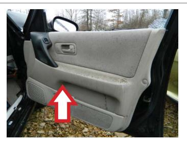
**STEP 14:** Verify that all of the interior door trim panel attaching hardware is secure and that the window regulator is operating properly.
