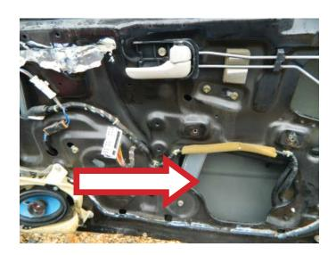
STEP 16: Remove the three window lift motor attaching screws.
