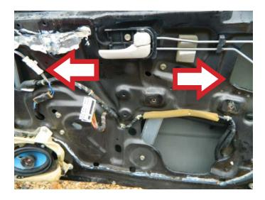
**STEP 10:** Once the window glass has been disconnected from the window regulator, manually slide the window glass into the closed position and hold in place with either a saddle cup assembly, painter's tape, or a wedge.
