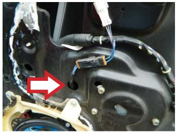
**STEP 13:** Using your ratchet with a 10 mm socket, remove the three screws that attach to the window regulator assembly.
