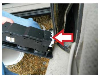
**STEP 11:** Attach the power window switch assembly onto the interior door trim panel. **NOTE:** Your vehicle switch may vary in appearance depending upon which options you vehicle came with.
