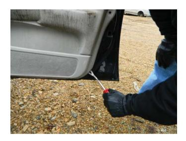
**STEP 6:** To remove the interior door trim panel, pull the interior door trim panel toward you and lift in an upward motion.
