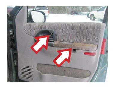
**STEP 2:** Remove the master switch assembly by using either your plastic pry tool or a flat-blade screwdriver.
