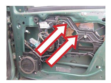
**STEP 9:** Remove the glass attaching bolts from the door glass.
