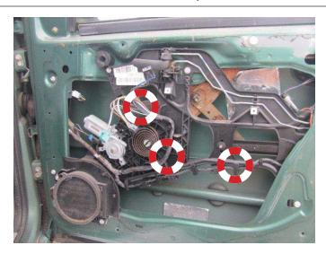
**STEP 7:** Remove the speaker using a 10mm socket.
