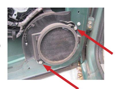
**STEP 7a:** Disconnect the speaker assembly and remove.
