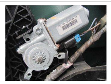
**STEP 8a:** Disconnect the door handle latch rods from the window regulator door module.
