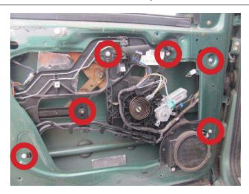
**STEP 10:** Remove the window regulator module assembly.
