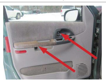
**STEP 15:** Install the power master door switch assembly.
