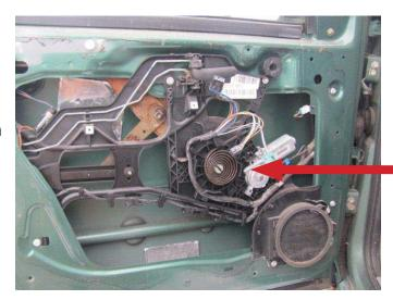
**STEP 6:** Disconnect the electrical connector at the window lift motor.
