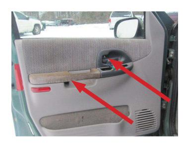
**STEP 2:** Remove the master switch assembly by using either your plastic pry tool or a flat-bladed screwdriver.
