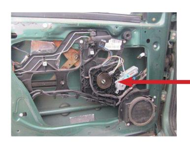
**STEP 5:** Attach the window regulator door assembly onto the door.
