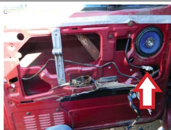
**STEP 6:** Using a ½" drill bit and a power drill, drill out the two (2) rivets holding the door brace onto the door. **NOTE:** You are using the drill and drill bit to remove the head of the rivet. DO NOT DRILL ALL THE WAY THROUGH. YOU WILL DAMAGE THE DOOR AS WELL AS THE BRACE.
