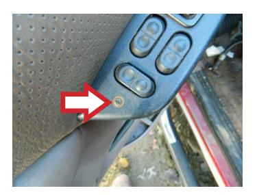
**STEP 12:** Verify that all of the interior door trim panel attaching screws are mounted securely and that the window is operating properly.
