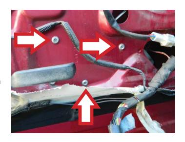
**STEP 9:** Remove the window regulator through the access hole.
