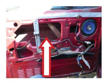
**STEP 2:** Install the window regulator onto the door and connect the window lift motor connector. **NOTE:** If you do not have access to a large rivet gun capable of handling ¼" x ¾" rivets, it is okay if you use ¼" x 20 x up to 1" bolts washers and the corresponding nylon locking nuts when installing the window regulator onto the door.
