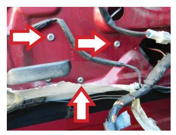
**STEP 3:** Once the window regulator has been installed, manually lower the window glass into position to attach onto the window regulator.
