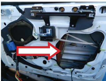
STEP 14: Remove the three (3) window lift motor attaching bolts.
