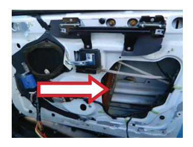
**STEP 2:** Using Dorman installation kit 702-013, attach the window regulator assembly to the door. **NOTE:** The Dorman installation kit 702-013 is comprised of 1/4" X 1" bolts, 1/4" nuts, and 1/4" washers.
