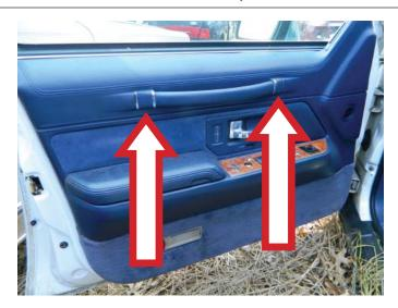
**STEP 12:** Verify that the window regulator assembly is operating properly and that all of the interior door trim panel retaining screws are tight.
