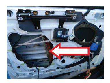
**STEP 2:** Using Dorman installation kit 702-013, attach the window regulator assembly to the door. **NOTE:** The Dorman installation kit 702-013 is comprised of 1/4" X 1" bolts, 1/4" nuts, and 1/4" washers.
