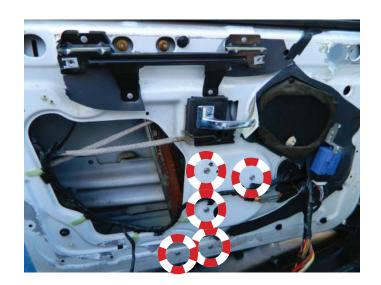
**STEP 12:** Remove the two (2) window regulator attaching nuts.
