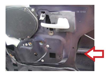
**STEP 2:** Install the window regulator assembly through the access hole.
