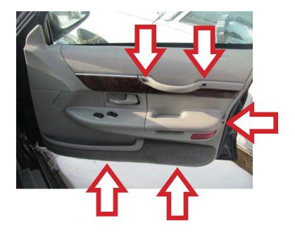
**STEP 2:** Using a trim panel removal tool, gently pry-up the master switch assembly.
