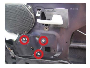
STEP 4b: Attach rivets.
