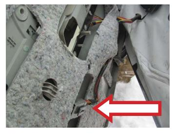
**STEP 9:** Install the door trim panel, making sure that all mounting holes are aligned. Be sure to pull the master switch wiring through the door trim panel.
