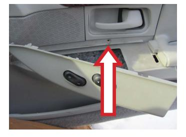
**STEP 4:** Making sure that all of the door trim panel screws have been removed, lift the door trim panel in an upward and outward movement.
