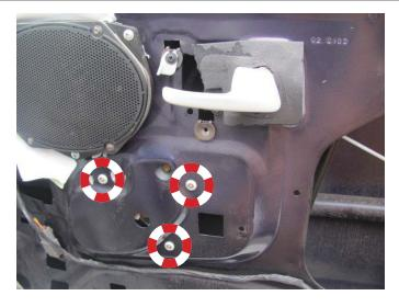
**STEP 12:** Remove the bolts that attach the window glass to the regulator.
