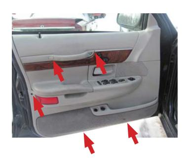
**STEP 2:** Use panel retainer remover to carefully pry-up the master switch assembly.
