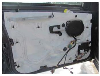
**STEP 7:** Attach the courtesy lamp connector.
