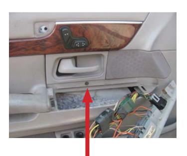
**STEP 5:** Once all of the door trim panel screws have been removed, lift the door trim panel in an upward and outward movement.
