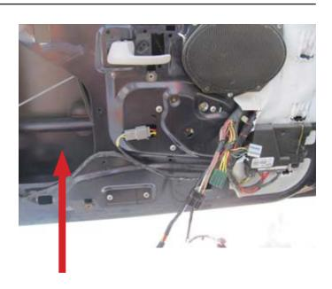
**STEP 15:** Remove the three (3) screws attaching the window lift motor to the window regulator.
