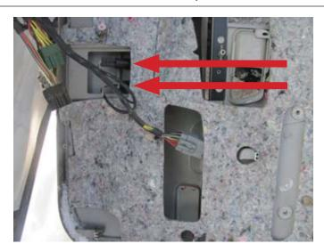
**STEP 8:** Install the door trim panel, making sure that all mounting holes are aligned. Be sure to pull the master switch wiring through the door trim panel.
