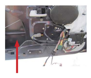
**STEP 2:** Attach the three (3) Torx screws that attach the window motor assembly to the door assembly.
