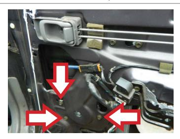
**STEP 13:** Remove the window regulator assembly through the main access hole. **NOTE:** At this point, your interior door trim panel reinforcement bracket would be removed.
