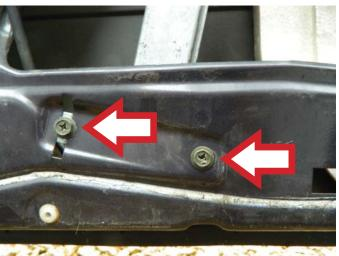
**STEP 4:** Tighten down the window lift motor attaching hardware.
