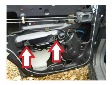
**STEP 7:** Remove the water vapor barrier.
