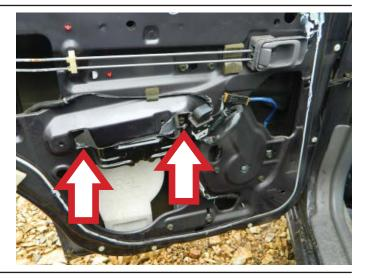
**STEP 9:** Install the interior door trim panel. **NOTE:** When installing the interior door trim panel, pull the door trim panel in a downward motion. Be sure to align the door trim panel on the lip of the door and align the interior door trim panel retaining hardware with its corresponding holes. Once everything is aligned, press the interior door trim panel into position.
