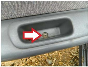
**STEP 12:** Attach the interior door trim panel attaching screws.
