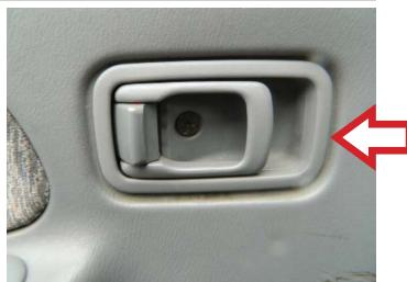
**STEP 5:** Using a trim panel removal tool, place the tool between the door and the interior door trim panel and using firm, even pressure release the interior door trim panel from the door.
