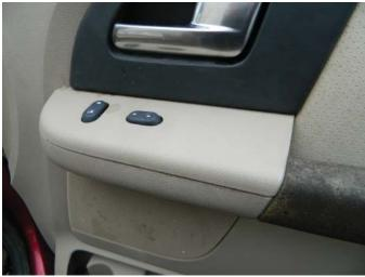
**STEP 15:** Install the power switch assembly.
