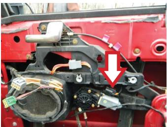
**STEP 12:** Disconnect the window lift motor connector.
