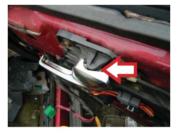
**STEP 10:** Temporarily connect the window switch to lower the door glass, exposing the two (2) bolts mounting the door glass to the window regulator. You will be using a 10mm socket with extension and a ratchet.
