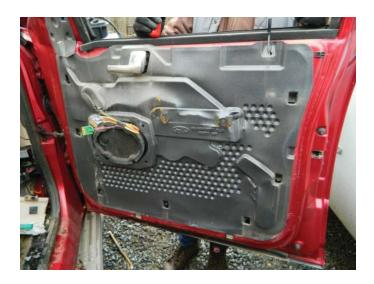
**STEP 10:** Attach the water vapor barrier.
