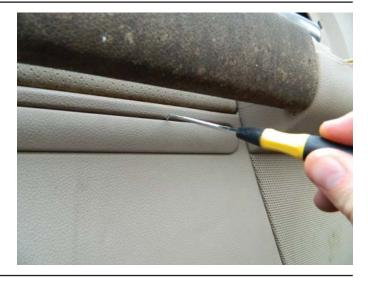
**STEP 19:** Install the interior door trim panel retaining screw cover.
