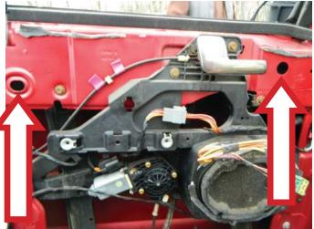
**STEP 11:** Once the door glass has been separated from the window regulator, manually slide the door glass into the closed position and hold in place with a saddle cup assembly, painters tape, or a wedge.
