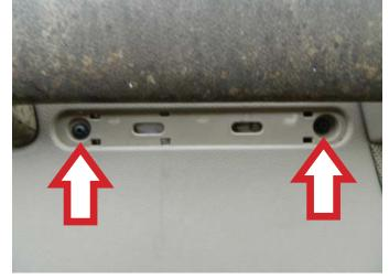
**STEP 7:** Once all of the interior door trim panel retaining screws have been removed, lift the interior door trim panel in an upward and outward motion to remove the panel.
