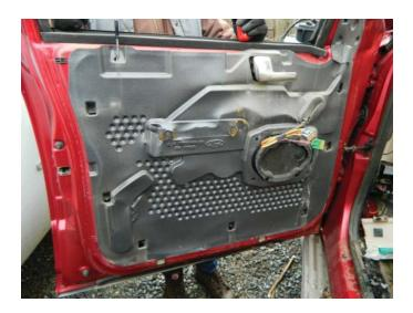
**STEP 10:** Attach the water vapor barrier.
