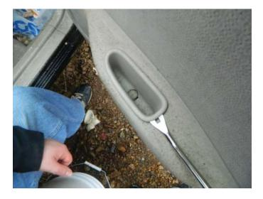
**STEP 3:** Using your trim panel removal tool, remove the door pull cup assembly.
