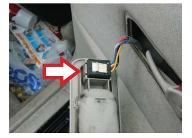
**STEP 11:** Attach the power window switch assembly onto the interior door trim panel. **NOTE:** Your vehicle switch may vary in appearance depending upon which options you vehicle came with.
