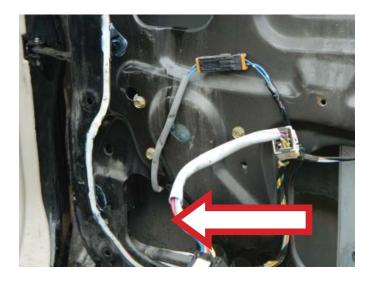
**STEP 2:** Slide the window lift motor connector through the access hole.
