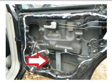
**STEP 17:** Remove the three window lift motor attaching screws.
