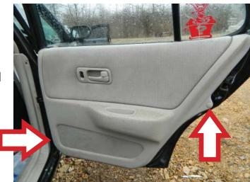
**STEP 6:** Remove the interior door trim panel retaining screw covers and the interior door trim panel retaining screws.
