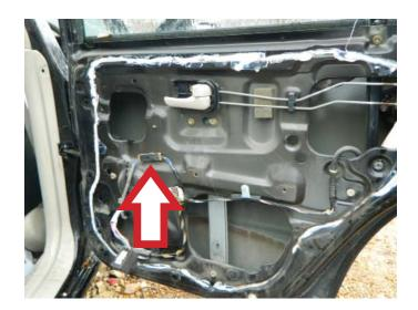
**STEP 13:** Push the window lift motor connector through the access hole in the door.
