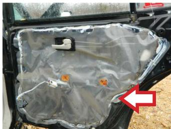
**STEP 9:** Remove the water vapor barrier.
