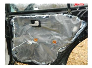
**STEP 7:** Install the water vapor barrier.
