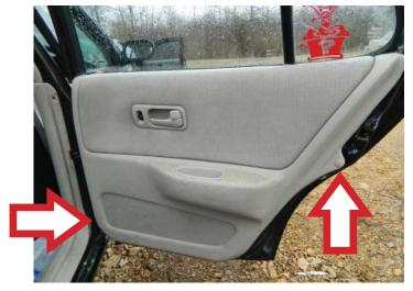
**STEP 2:** Using a trim panel removal tool, remove the screw cover for the door handle pull assembly and the door handle pull assembly retaining screw.
