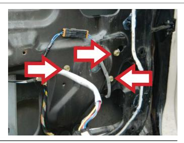
**STEP 15:** Using your ratchet with a 10 mm socket, remove the remaining window regulator attaching hardware.
