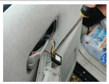
**STEP 6:** Remove the interior door trim panel retaining screw covers and the interior door trim panel retaining screws.
