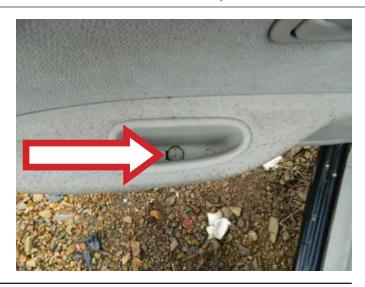
**STEP 13:** Attach the door handle pull attaching screw. Install the screw cover assembly.
