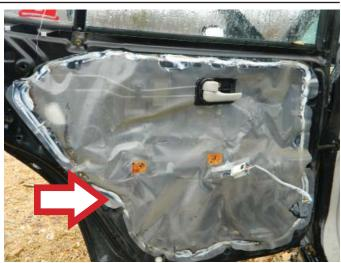
**STEP 10:** Temporarily install the window switch to lower the window glass, exposing the window glass to window regulator attaching screws.
