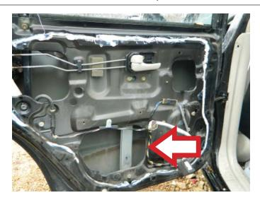
**STEP 17:** Remove the three window lift motor attaching screws.
