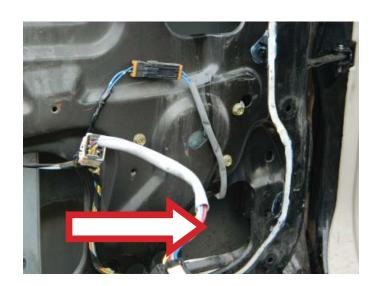
**STEP 3:** Connect the window lift motor connector.
