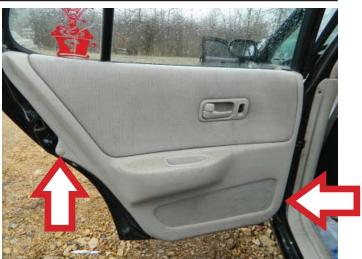
**STEP 7:** Using your trim panel removal tool, remove the interior door trim panel. Pull the interior door trim panel toward you and lift in an upward motion.
