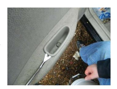
**STEP 4:** Using a trim panel removal tool, remove the interior door handle bezel assembly.
