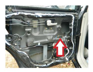
**STEP 13:** Push the window lift motor connector through the access hole in the door.
