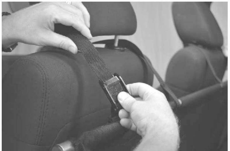
Now you can connect the snaps down the side on to the structure-d-rings you installed earlier. The tail end of the liner should line up with the end of the bed and hook and loop fastener down to the carpet.
