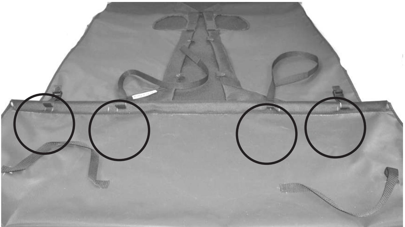
Once the bar is in place you can put the liner in place with the back seats down. (Once this installation is done we will show you how install it with the back seats up.) There are two straps sewn to the back side of the cargo liner. These two straps loop around the rear seat head rest as shown. The two straps around the top go around the front seat head rest and connect to the cam lock.
