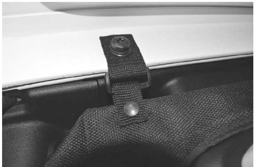
To install the door /bumper protector you must clean the uoY .tsrfi ecafrus rood edisni will need to stick the 3 adhesive hook and loop fasteners to the door as shown. Use the door protector piece to line up where the hook and loop fastener is positioned. Use the alcohol wipes to clean the area where the adhesive hook and loop fasteners will be attached.
