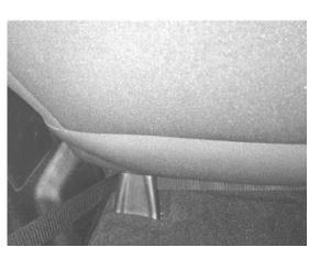
On the 2 dr wrangler you will have to reach a little further under the seat to feed the strap underneath as shown
