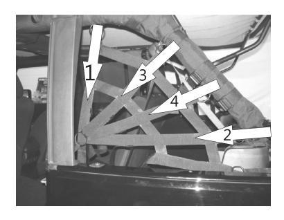
The last strap at the bottom can now be installed using the loop at the rear strap that you installed at the beginning.
