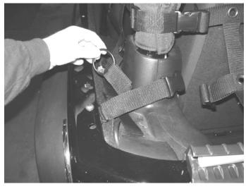
Slide each half of the tailgate bar in the last row as shown in the photo. This bar will connect at the center of the net and then the whole bar is clipped into soft-top tailgate clips. (Clips can be purchased form us or your local dealer.) This last row is optional and can be cut off if not needed.
