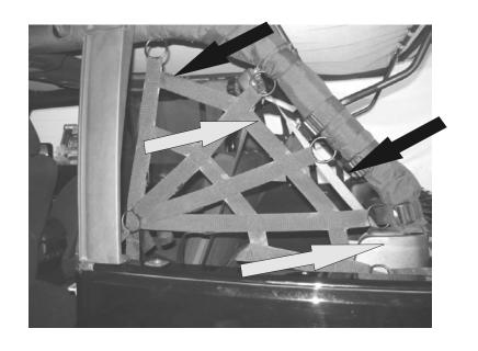
Next is to install is the attaching strap with the nut and washer provided. This is the strap that has a single ring on one end. This attaches to the existing bolt stud that you will find under the carpet directly behind the rear door
