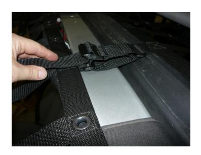
The final will be to install the shock cords around the footman loops at the top of the windshield as shown
