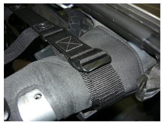
The next step is the rear corners. You need to take the long straps and feed them in between the roll bar and the sound bar. You may need to loosen of the sound bar bolts temporally so you can push the strap through. These bolts are found on the underside of the sound bar. Pull it through the bottom and up around the outside of the roll bar and connect to the ladderloc on the top again. Do this on both sides. Go around and adjust the net so the piece is centered on top.
