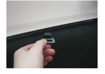
Slide the top straps through the slot in the plastic hook and tighten. Do this on both sides. Your barrier is now installed.
