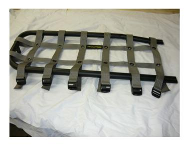
TURN THE DOOR OVER AND PUT THE LOOSE END OF THE STRAP THROUGH THE LADDER LOC BUT **DO NOT TIGHTEN THE STRAPS** AT THIS TIME. THE DOOR MUST BE INSTALLED FIRST AND THEN THE STRAPS CAN BE TIGHTENED UP. FOLLOW THIS PROCEDURE FOR EACH DOOR.
