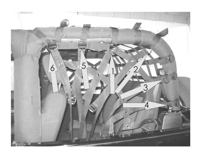
Find the strap that has a metal ring and a plastic loop installed on one end and hook and loop fastener sewn to the other end. This strap is installed on the roll bar beside the seat. The strap wraps around the roll bar passes through the plastic loop and the hook and loop hooks onto itself. Be sure that the strap gets pushed below the body side so it falls below the padding of the roll bar. The ring should pull out toward the back.
