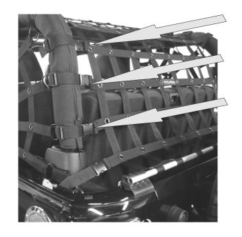
The next three straps heading toward the top can now be installed. They have laadderlocs already sewn into the net. The net is positioned properly when the top strap is installed directly behind the speaker bar. (pictured with standard sides)
