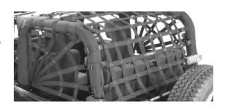
You can now skip the next two straps and go to the final straps at the front corners. These straps wrap over the speaker bar. Wrap the long strap around over the front of the speaker/roll bar and bring under and around up the side and feed into the ladderloc. There will be two ladderlocs. The second one is used for the side strap. See photos next page
