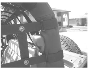
The four straps at the top of each side will connect to the top piece after you have installed the overhead piece.
