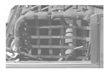
The next step is to install the back side. Start at the back and install the 8 buckles.
