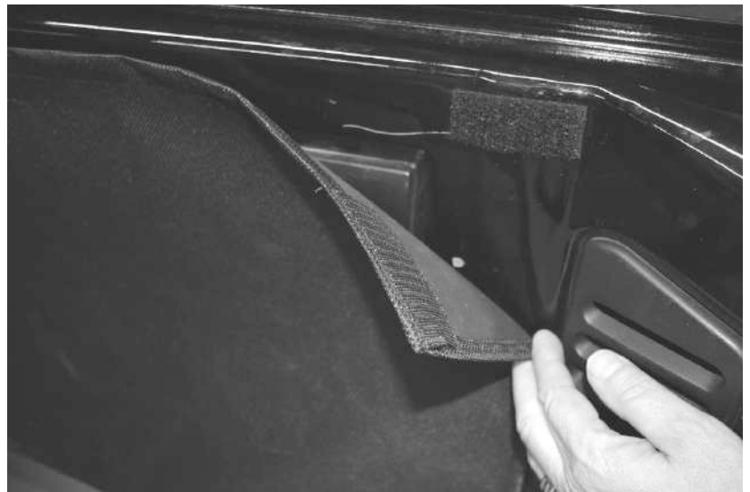
self adhesive hook and loop fastener
