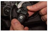
4. Plug the SL1 connector into the factory electrical socket.
