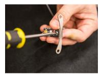
1. To begin, attach the Demon Eye to the top of the included bracket, using one of the included locking screws and locknuts. Ensure the locknut is on the bottom side of the Demon Eye. Be sure to thread the locking screw and locknut first and then tighten using pliers and a small Philips screwdriver.
