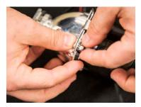
2. Next, mount the Demon Eye inside the projector housing, ensuring the Demon Eye board is inside the shroud. The bracket can be mounted on either the front or the back side of the projector housing. Using the mounting holes and included locking screws, secure both sides of the bracket to the housing. Again, thread the locking screws and locknuts and then tighten using pliers and a small Philips screwdriver.
