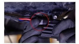
14. Plug the DT connector into the back of the pods and the amp connector into the provided universal harness coming from the taillight ①.
