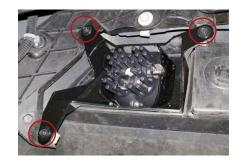
4. Install your assembled bracket and pod onto the vehicle by securing the three original bolts with a 7mm socket and ratchet.
