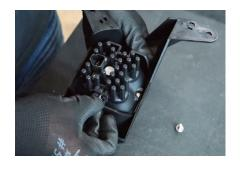
1. Install the supplied nuts into the pod housing with the nylon facing inward. Attach the bracket to the pod using the supplied screws and washers. Make sure the bracket is in the correct orientation. See diagrams above. Ensure that the screws are tightened such that the pod retains its position, but can pivot with force for aiming.
