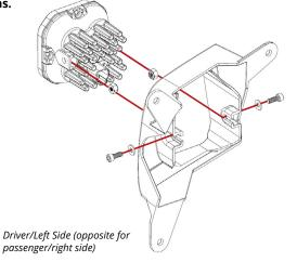
3. Use a 7mm socket and ratchet to remove the three bolts holding the factory fog light housing in place, as shown in the picture to the left. Remove the factory fog light housing. The factory bolts will be reused.
