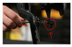
8. Reinstall the adjustment screw, spring, and plastic clip to the bottom of the bracket.
