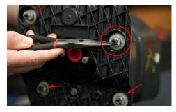
3. Set the foglight bracket assembly on a table. Remove the four metal retaining washers using a pick or flathead screw driver. Then remove the four 13mm nuts that secure the front bezel to the foglight bracket.
