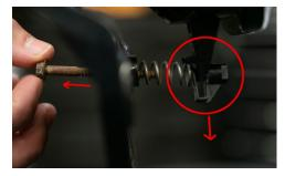
4. Remove the adjustment aiming screw using an 8mm socket.
