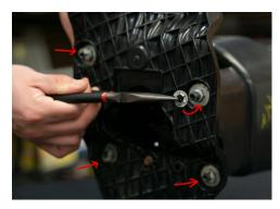
10. Reattach the metal retaining washers.
